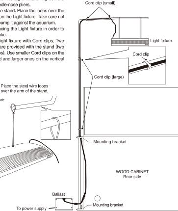
\*The ballast can be installed inside WOOD CABINET.
